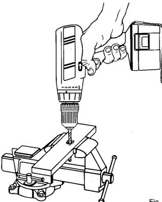
Move the drill bit into the workpiece applying only enough pressure to keep the bit cutting. Do not force or apply side pressure to elongate a hole.
